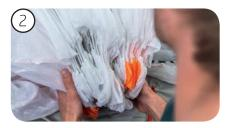
Lay the Rigid Foils of the leading edge on top of one another. It's best to start from the middle and work on one half of the glider, then do the second half and place its Rigid Foils next to those of the first half.
