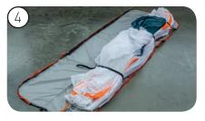
Now sort the rest of the glider lengthwise to the trailing edge and fix it with the remaining compression bands.
