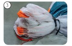
Turn the entire leading edge 90° on its side and fix the glider with the first compression band to the Softbag.
